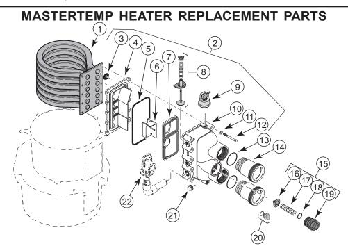
**REPAIR PARTS – WATER SYSTEM**
