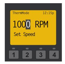
Setting the Thermal Mode Pump Speed
