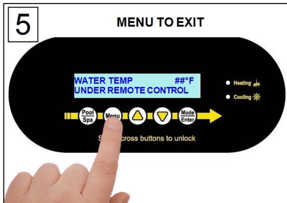
10. If after 45 seconds, the heat pump displays a "**SMART COMM FAULT**":
