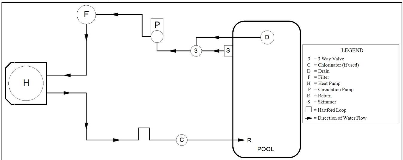
**Heat Pump with water flows greater than the maximum listed flow rate**
