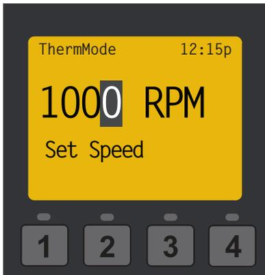
Setting the Thermal Mode Pump Speed
