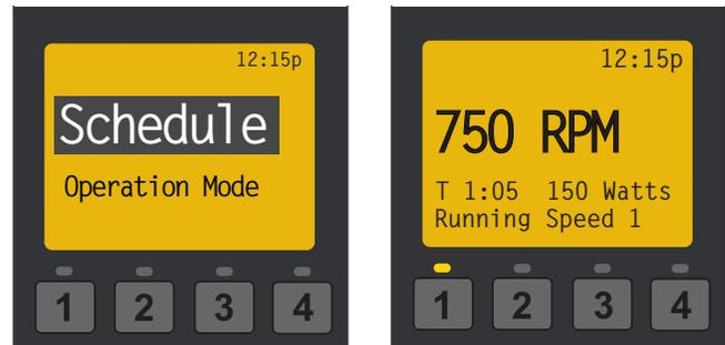
**Note:** The pump will not run the scheduled speeds or flows until the **Start/Stop** button is pressed (LED on) to place the pump in Schedule mode.
