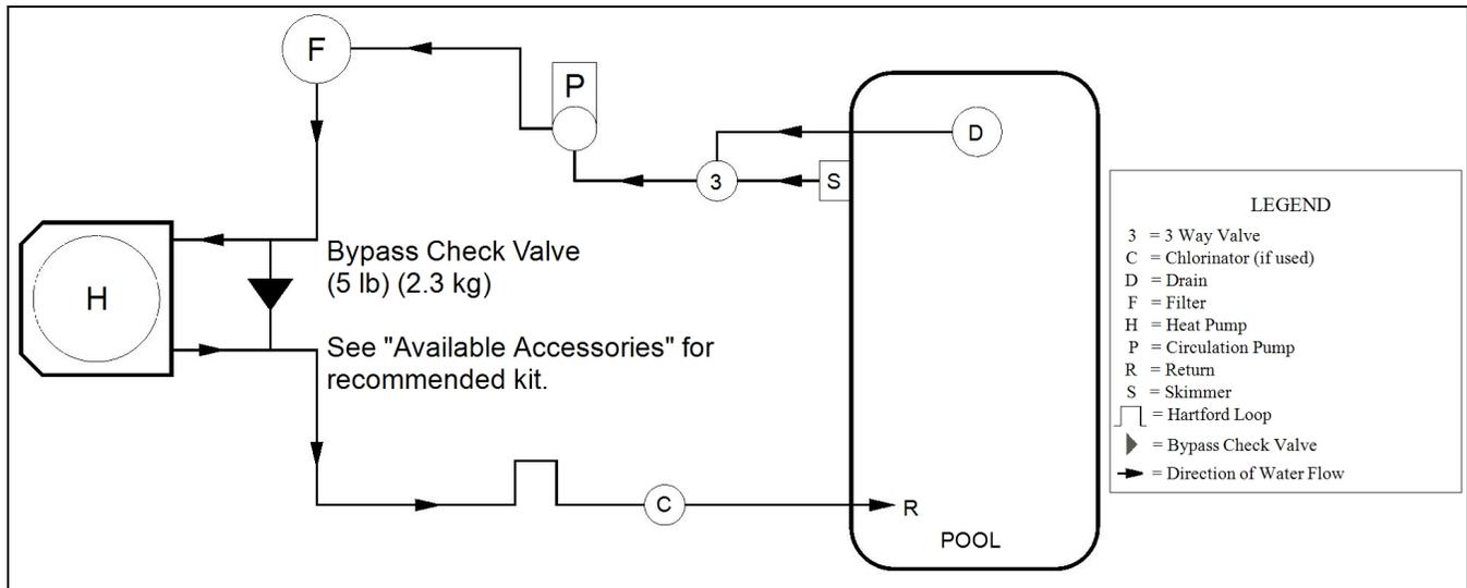
**Heat Pump with Spillover Spa (One filter Pump)**
