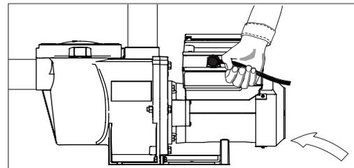
4. Reinstall the RS-485 communication cable.
