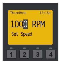
Setting the Thermal Mode Pump Speed
