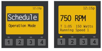
**Note:** The pump will not run the scheduled speeds or flows until the **Start/Stop** button is pressed (LED on) to place the pump in Schedule mode.
