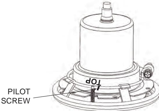
10. **Aligning the face ring and lens:** Align the face ring and vertical line on the lens so that the letter "O" in the word "TOP" and the small arrow above it) on the surface of the lens points to the 12 O'clock position and with pilot screw hole on the face ring.
