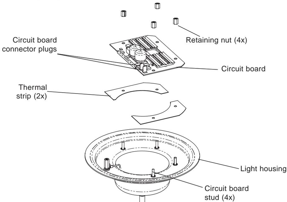
4. Place the two new thermal strips (provided) over the circuit board studs in the base of the light housing.
