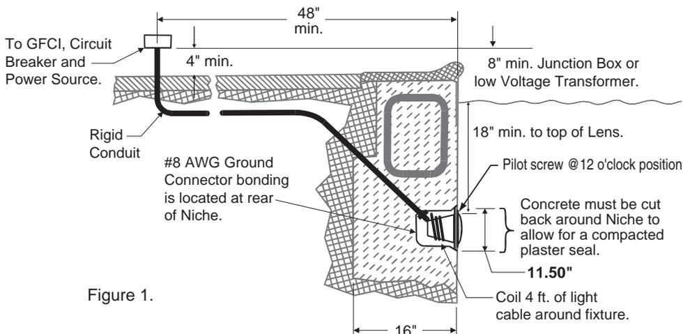
2. Cut the cable at the Junction Box, leaving at least six (6) inches (2.4 cm) of cord to make connections.
