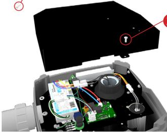
3 Remove single screw to electrical enclosure cover.
