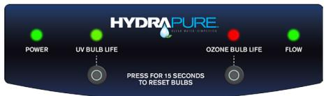
Solid red OZONE BULB LIFE indicates malfunction with ozone bulb and should be replaced immediately, see page 13
