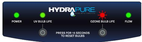
Red flashing OZONE BULB LIFE indicates ozone bulb no longer producing ozone and should be replaced soon, see page 13
