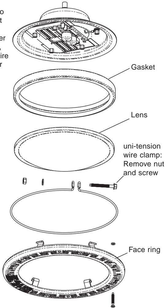
Note: Note the current position of the lens at the pilot screw (12 o'clock) position, before removing it from the fixture. "W" on the lens indicates wide angle, "N" indicates narrow angle. For more information, see page 17.
