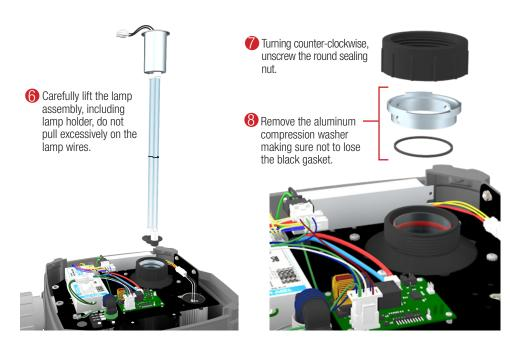
**NOTICE:** Do not touch the glass part of the lamp as body oils will create hot spots & greatly shorten lamp life. Inspect the quartz tube carefully for any cracks or chips and replace the quartz tube if any are found. Do not use any other O-ring for sealing the quartz tube. Never use any type of lube or sealing agent. Doing so can result in a leak and possibly damaging the UV unit.
